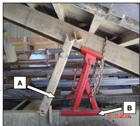
This picture shows both the original manufactured body props (A) and a custom manufactured brace (B). The custom braces have handles which allow the worker to place the braces under the dump box without putting their body under the dump box.
